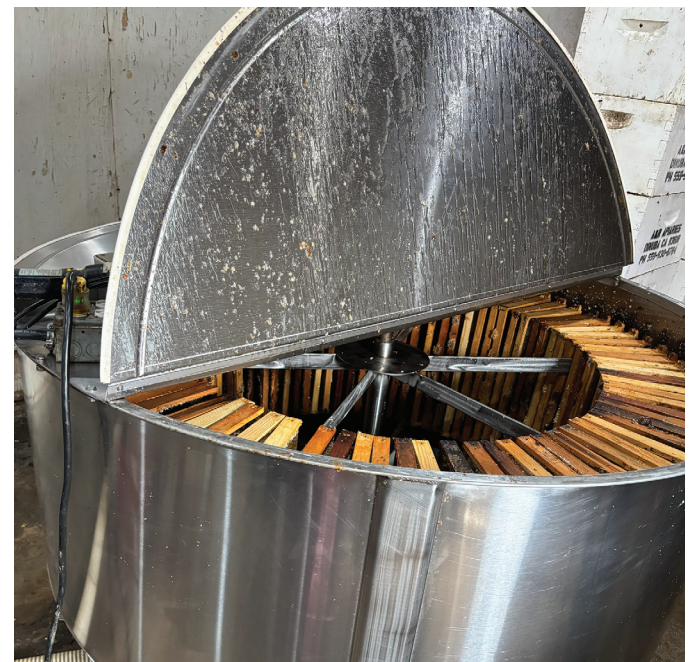
The honey extractor machine helps remove honey quicker from the frames. It holds up to 80 frames at a time.
